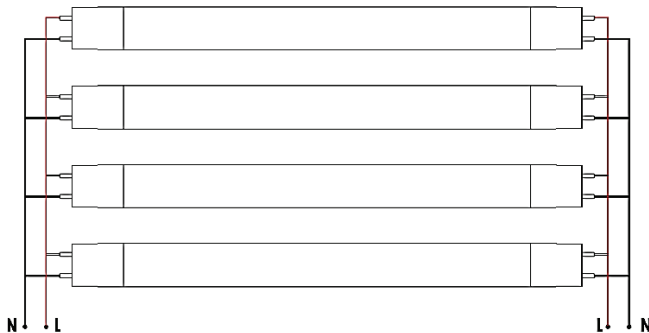
DSEP Wiring Diagram (6' & 8' T-Lites only)
